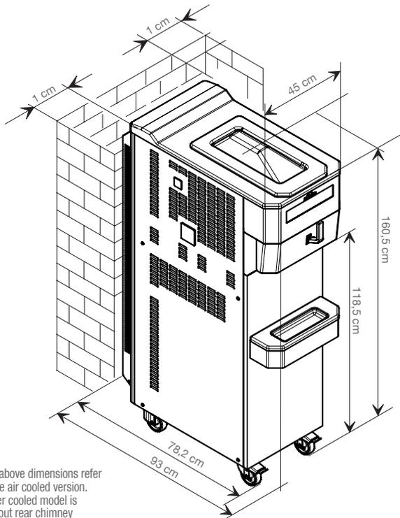
The above dimensions refer to the air cooled version. Water cooled model is without rear chimney
